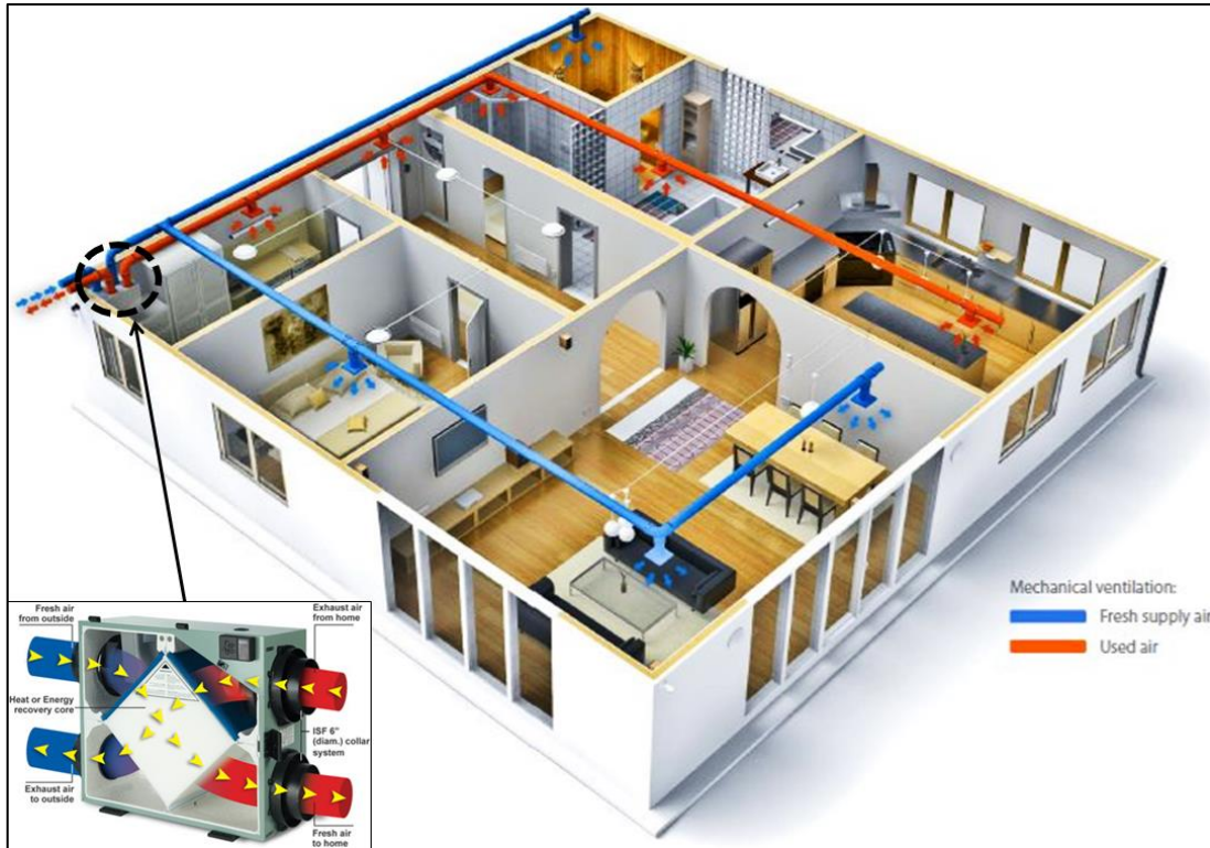
Figure 4: Balanced Whole house Mechanical Ventilation with heat recovery
